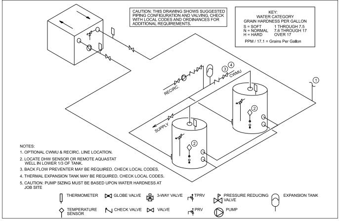
Figure 11. Water Heater Piping — One Heater, Multiple Tanks.
